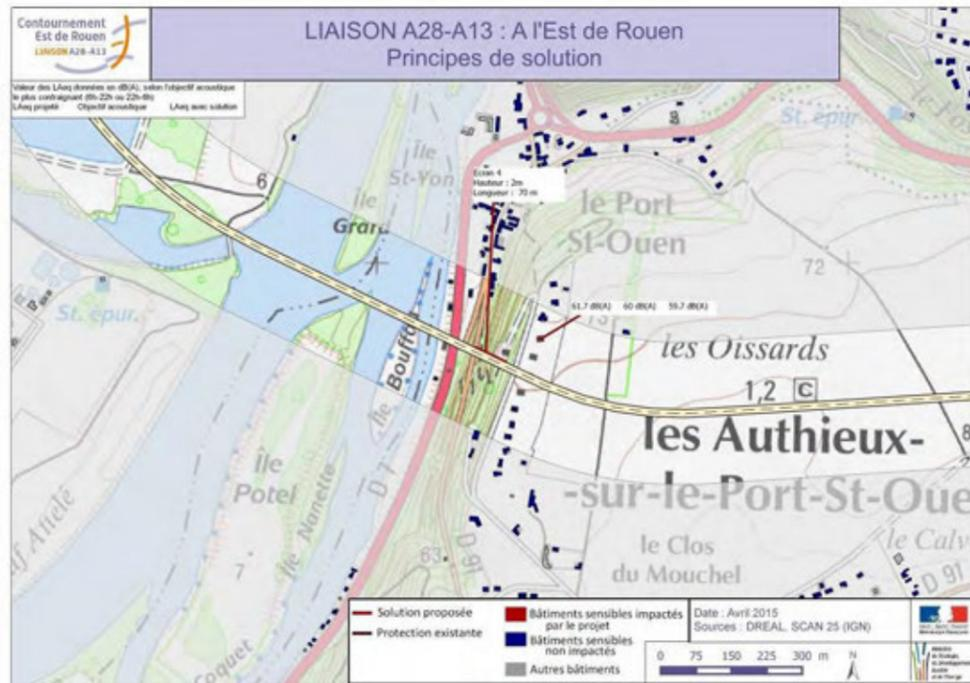
FIGURE 327 PRINCIPE DE SOLUTION PHONIQUE DANS LA ZONE DU VIADUC [GAMBA]
